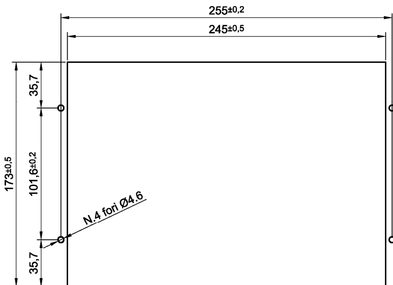
Dima montaggio da incasso Flush mounting panel cut-out
